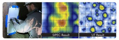
SIPECTM Dynamic Pulsed Eddy Current Inspections through Coating/Buildup
