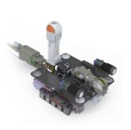
Robototic Tank Inspection Vehicle
