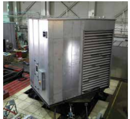
Air Handling Unit Awaiting Seismic Testing
