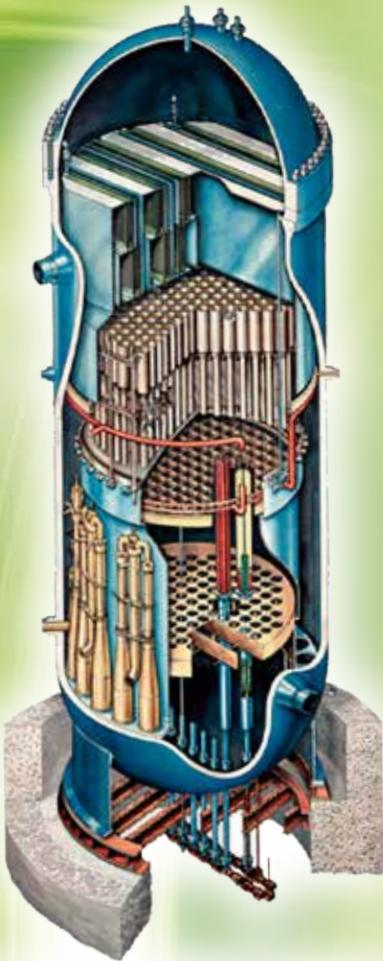
Figure 1: Typical BWR configuration illustrating annulus with shroud and jet pumps.
