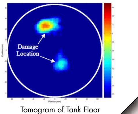
Figure 3. Example CT image showing the location and relative size of damage which has occurred in the tank floor.
