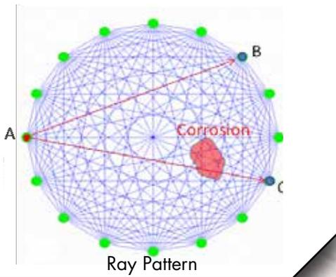
Figure 2. Ray pattern showing all unique combinations of transmitter-receiver sensor pairs.
