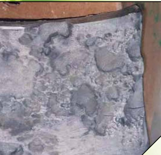
1. Sandblasted 10-Inch 40-Year-Old Cast Iron Pipe With Crack At Failure Location
