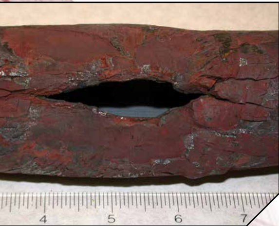
Failed superheater tube (long-term overheating)
