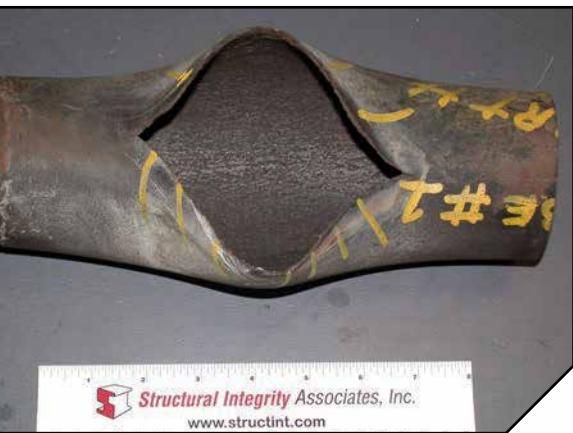
Failed waterwall tube (short-term overheating)
