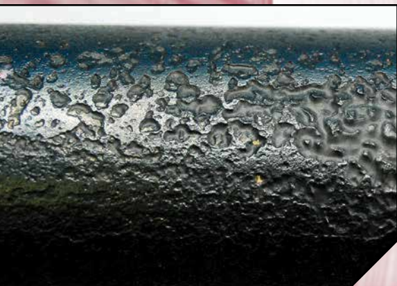
OD wastage on an economizer tube.
