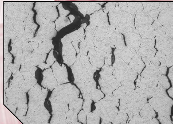
Creep in stainless steel reheater tube.
