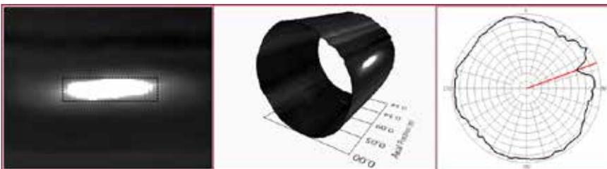
**Figure 4** Zoomed in C-scan display (left), rolled pipe C-scan display (middle), and cross-section view (right) of the 42-inch diameter pipe OD flaw.
