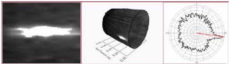
**Figure 2** Zoomed in C-scan display (left), rolled pipe C-scan display (middle), and cross-section view (right) of the 42-inch diameter pipe ID flaw.
