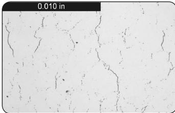
Figure 2 Volumetric Grain Boundary Graphitization
