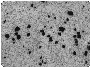
Figure 3 Typical Graphitization in Low Alloy Steel
