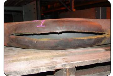
Figure 1 PSH Piping Failure
