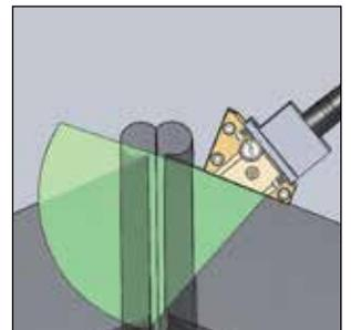
**The technique developed by Structural Integrity Associates, Inc. is optimized to examine up to 7 inch wall-thickness.**
