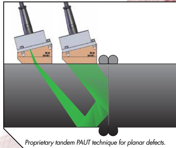
Proprietary tandem PAUT technique for planar defects.
