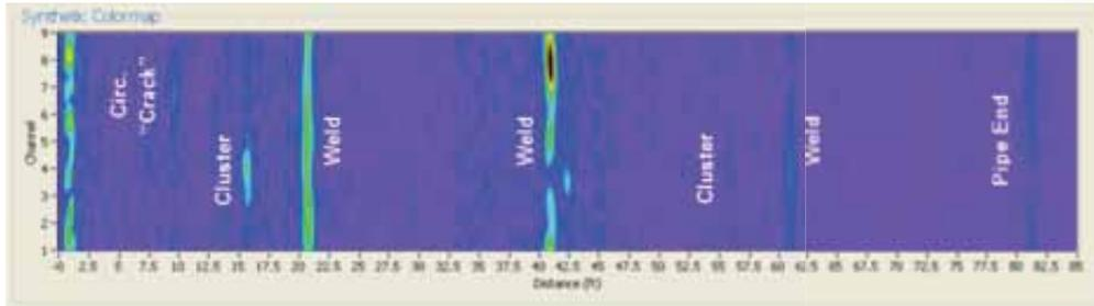
Pipe "image" generated using the Total Focal Scan™ capability of the PowerFocus™ system with the MEF sensor.
